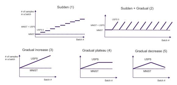
Figure 2: Unstructured datasets with various types of drifts.
