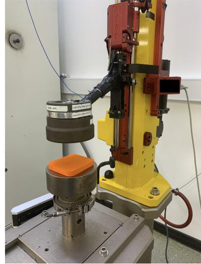
Fig. 2. Image of the Cadex drop tower used for experimental data collection for the 98A data set.
